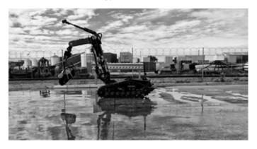
With two independently operated arms (one for the claw and one for disruptors), the robot can easily pick up large items and disrupt them in a safe area. ICOR designed the robot for Large Vehicle Borne Improvised
